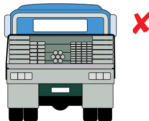
A load with substantial gaps that would allow potentially dangerous movement.
