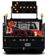
Lit arrow sign on vehicle or at the side of the road (road hazard ahead, merge into another lane)
